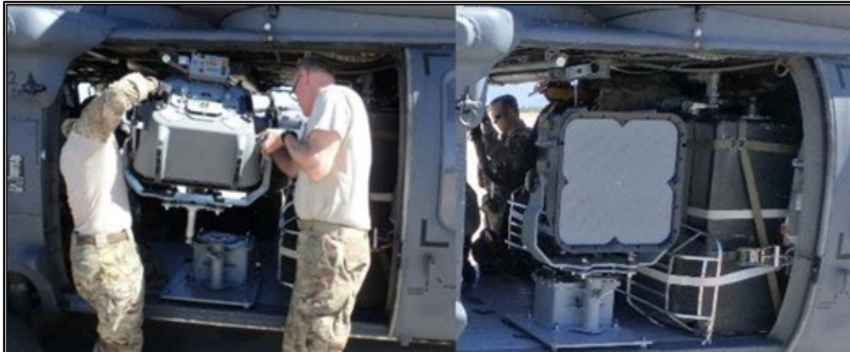
Figure 4-7. The Long Range Acoustic Device model 500x during test
